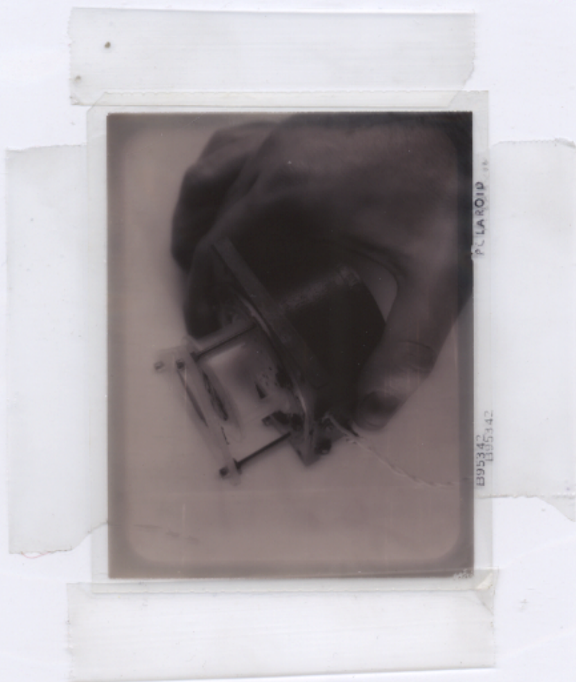
MOVING COIL MAGNETIC TRANSDUCER WITH ^{57}\text{Fe} SOURCE & ARNCO IRON FOIL ABSORBER FROM W.W. II FM ALTIMETER
