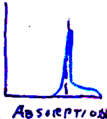
Fig. 2. Difference in intensity of the 129-keV gamma transition in \text{Ir}^{191} measured behind a resonance absorber (iridium) and a comparison absorber (platinum). This intensity difference is plotted as a function of v , the relative velocity of the source with respect to the absorber. Both source and absorber are at a temperature of 88^\circ\text{K} . \Delta E = (v/c)E_0 denotes the energy shift of the 129-keV gamma rays.
