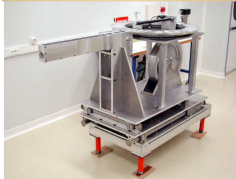
"Carousel" brick dispensing and storage system
