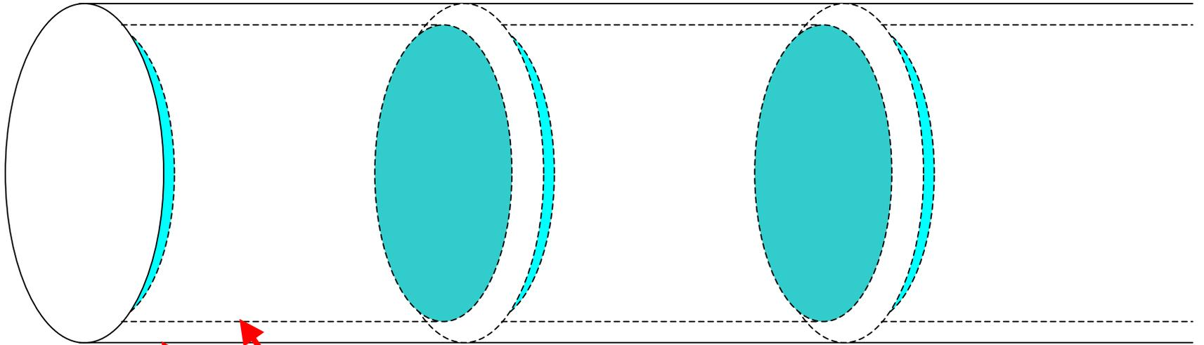
Fiducial volume:  $39\text{m } \phi \times 45\text{m} \times 10 \text{ sections}$
