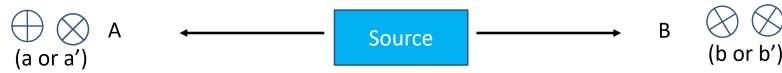
FIG. 1. Illustration of a source emitting pairs of photons. The circles with a cross are used to indicate the measurement axes.
