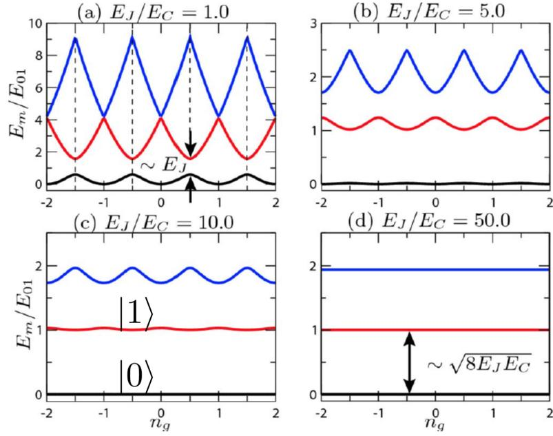
FIG. 8. Illustration of the energy levels of a transmons; pictures from Koch et al. [15].
