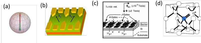
FIG. 2. Various qubit implementations with spins. (a) Bloch sphere of a spin, (b) Quantum dots, (c) Phosphorous donors on silicon, and (d) Nitrogen-vacancy centers in diamond.
