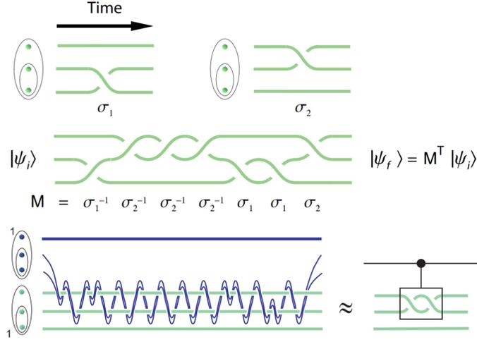
FIG. 14. Illustration of quantum gates in the Fibonacci model.
