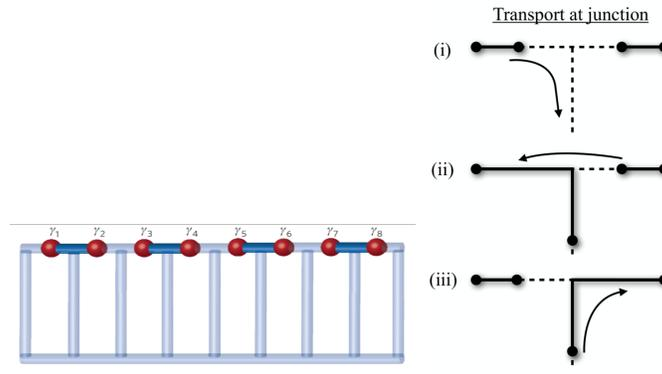
FIG. 18. Illustration of segments of Kitaev chain and braiding via the T junction; figures taken from Ref. [12].
